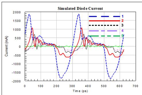
Fig. 3-(b) Simulated diode current; Pin=100W; freq=3.2GHz
