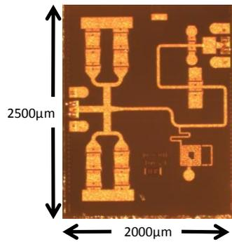
Fig. 7: Fabricated MMIC limiter
