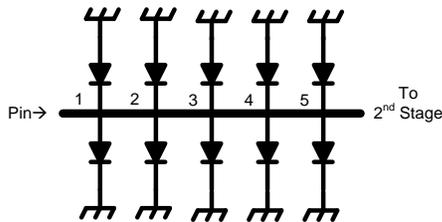
Fig. 2: Conventional limiter diode input string topology
