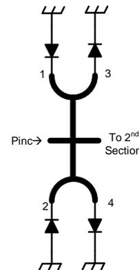
Fig. 4: New limiter input topology using binary splitters
