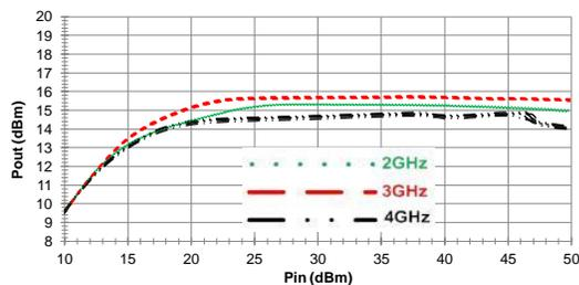
Fig. 9: In-fixture measured CW  $P_{in}$  vs.  $P_{out}$  at 2, 3, and 4GHz
