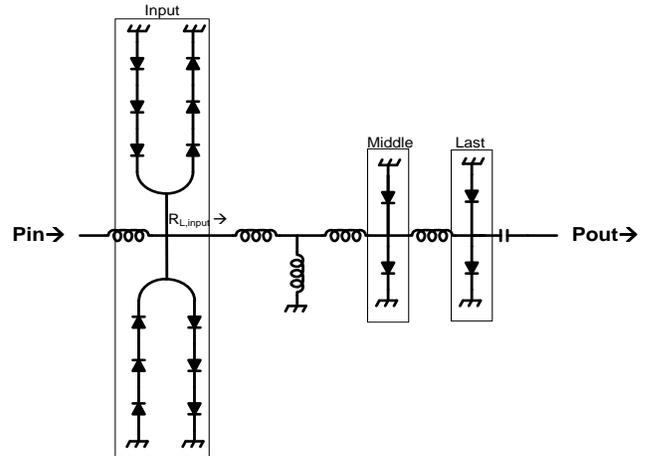
Figure 6 – Basis limiter schematic
