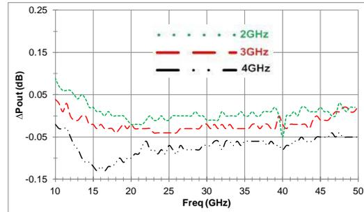
Fig. 10:  $\Delta P_{out}$  after 100W applied for 1 Hr.
