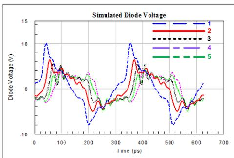
Fig. 3-(a) Simulated diode junction voltage; Pin=100W; freq=3.2GHz
