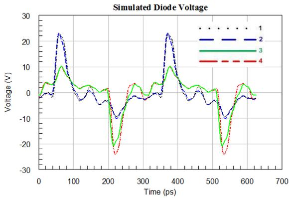
Fig. 5-(a): Simulated diode junction voltage;  $P_{in}=100W$ ;  $freq=3.2GHz$
