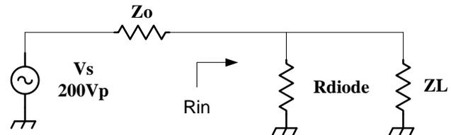
Fig. 1-(a) Equivalent circuit diagram of the limiter circuit
