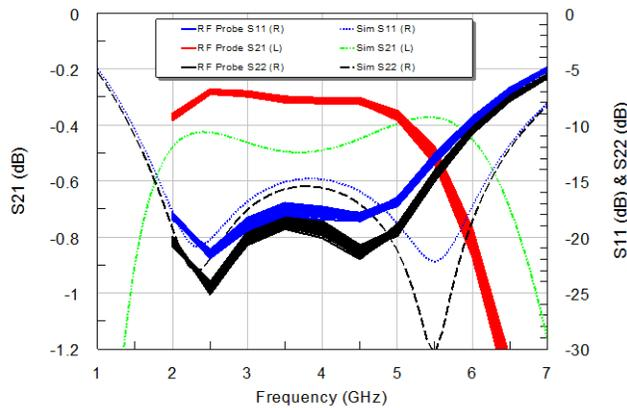
Fig. 8: RF Probe and Simulated IL, IRL, and ORL
